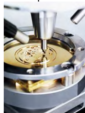
Figure 2.5: Microfabrication of watch components
