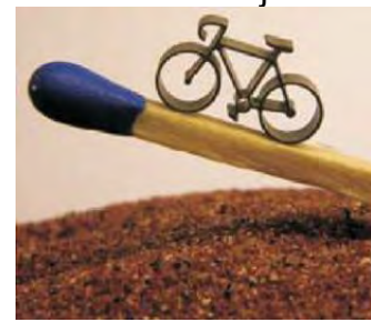
Figure 2.7: Examples of abrasive parts micro processed with water jet
