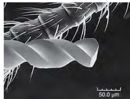
Figure 2.7: Examples of abrasive parts micro processed with water jet
