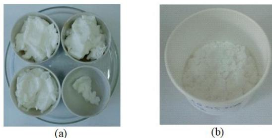
**Figure 7:** (a) Ag-CHAp before calcination; (b) Ag-CHAp after calcination
