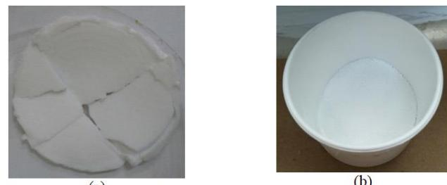
**Figure 5:** (a) CHAp before calcination; (b) CHAp after calcination
