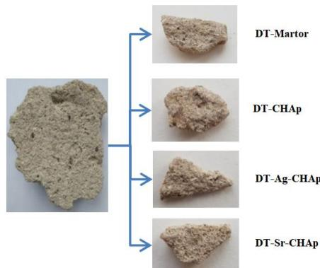
**Figure 46:** Samples from Corvins' Castel - Deserted Tower treated with CHAp, Ag-CHAp and Sr-CHAp
