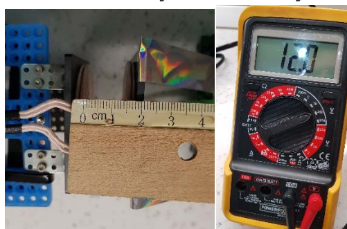
Fig. 93 1.5 cm distance between Tx and Rx coils and the value of the output voltage at the Rx module
