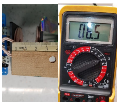
Fig. 95 The distance of 2.2 cm between the coils Tx and Rx and the value of the output voltage at the Rx module
